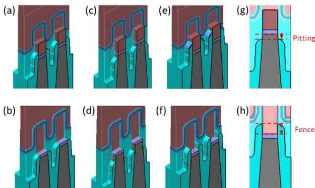
Figure 2. Pitting and fence defect. (a)-(b) Ideal etch structures post ONO etch and final etch, respectively. (c)-(d) Etch structures post ONO etch and final etch of pitting defect, respectively. (e)-(f) Etch structures post ONO etch and final etch of fence defect, respectively. (g)-(h) The schematics of AA pitting and fence measurement.
