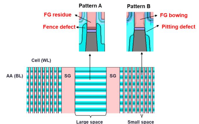
Figure 4. Pattern loading shown between patterns with different space. Pattern A with large space shows fence defect and FG residue issue; Pattern B with small space shows pitting defect and FG bowing issue.
