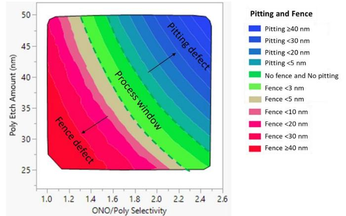
Figure 3. Contour map of ONO/Poly selectivity and poly etch amount at ONO etch step impact on final pitting and fence defect window of gate etch.
