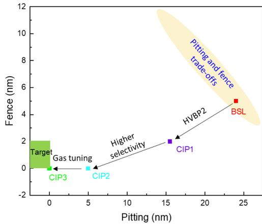
Figure 5. Process window optimization to break pitting and fence trade-offs.
