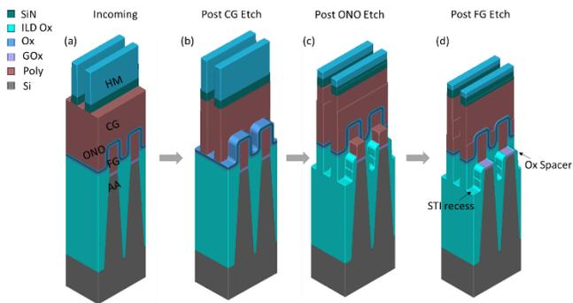
Figure 1. Schematics for the incoming film stack and by-step structure evolution of 2D NAND gate etch. (a) Post HM open. (b) Post CG etch; (c) Post ONO etch; (d) Post FG etch.
